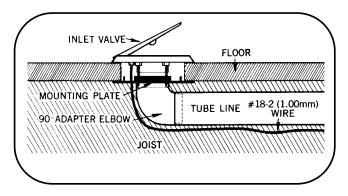
In the case of linoleum or uncovered floors, the mounting plate will be installed from below. If the floor is carpeted, cut a hole in the carpet with a utility knife and slip the untrimmed mounting plate under the carpet. Fasten the mounting plate to the floor with screws. If a wall or floor is over 1" (25 mm) thick, use inlet valve stem extension #5018. Shorten extension to fit. The flange on the extension should be 1/4" (6 mm) below the surface to insure a proper fit of the valve.
