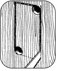
Having determined that there are no obstructions in the wall, cut a hole 2 1/4" (57 mm) wide by 3 3/4" (95 mm) tall for the inlet valve.
